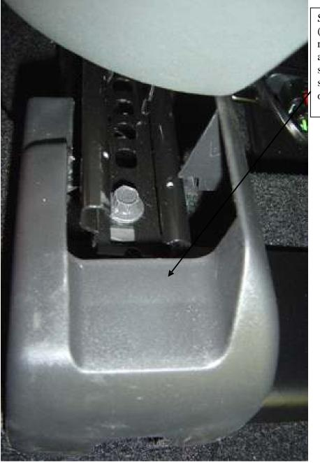
Seat Bolt Cover partially removed (VB129 Installed). This must be removed to gain access to the seat bolts and make room for the VB129. The seat track bolt is visible that mounts the seat track to the Load Cell Sending unit on the underside of the track.
