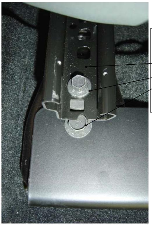
Here you see the bolt covers removed, and the VB129 installed on the forward mounting bolt of the load cell unit. The rear bolt of the load cell unit is not visible behind the track bolt.
